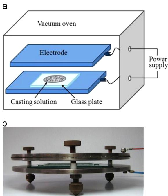
Fig. 1. Apparatus for electrical alignment of MWCNTs in polymer matrix. (a) A schematic and (b) a photo of the two electrodes and the glass plate.
