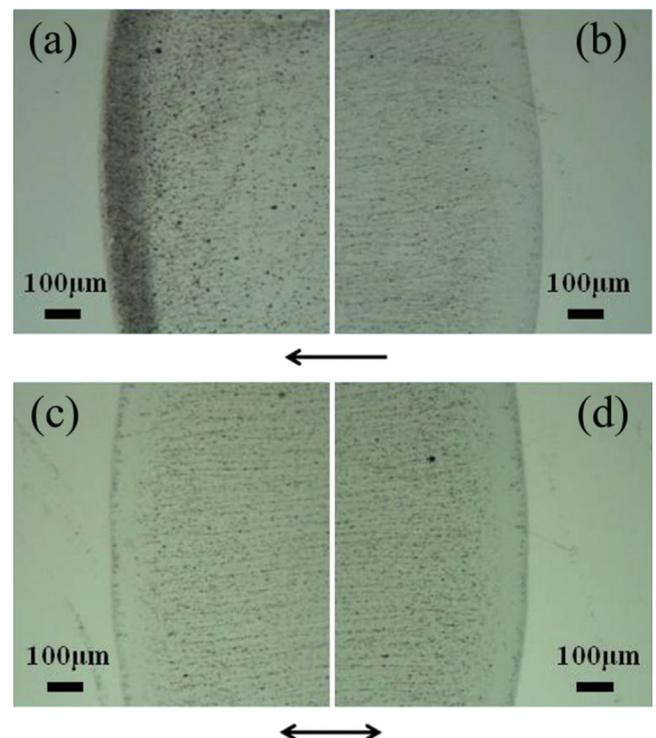
Fig. 3. Micrographs of local profiles of MWCNTs in a drop of 0.1 wt% MWCNTs casting solution near the two electrodes. The arrow indicates the direction of the electric field. (a) and (b): MWCNTs accumulate on the left side after migrating for 10 min along the direction of a 2000 V/cm static electric field; (c) (d): MWCNTs remain symmetrically distributed on both sides after exposing to a 2000 V/cm, 1 Hz alternating electric field for 10 min.
