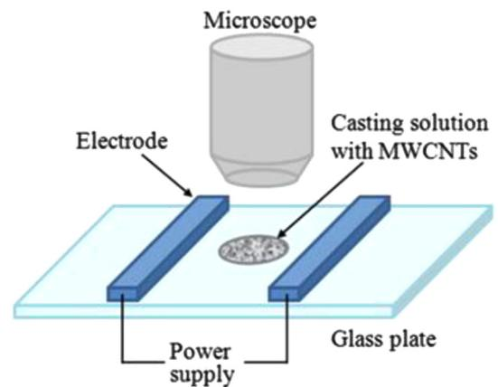
Fig. 2. Setup for observing the response of MWCNTs to electric field.
