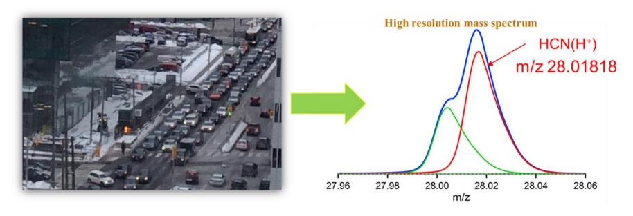
Laboratory and ambient measurements of hydrogen cyanide (HCN) from vehicles using high resolution Proton Transfer Reaction- Time of Flight- Mass Spectrometry (PTR-TOF-MS)
