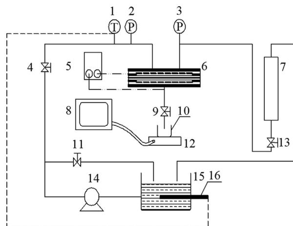
Fig. 1. Flow diagram of the coupling experiments. 1,16-device of controlling temperature; 2,3-pressure gage; 4,9,11,13-ball valve; 5-DC stabilized power supply; 6-membrane module; 7-rotameter; 8-computer; 10-beaker; 12-electronic balance; 14-pump and 15-feed.
