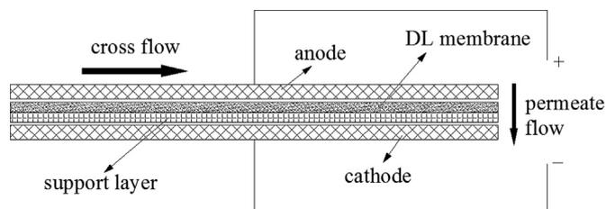
Fig. 2. Relative position of the electrodes and NF membrane in the membrane cell.
