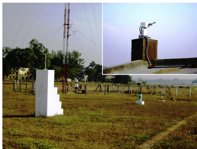
Fig. 1. Field view of micrometeorological tower with inset showing sun–sky radiometer installation.
