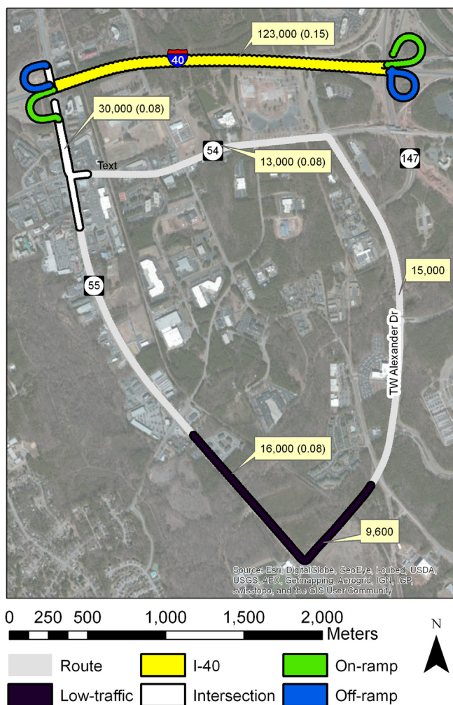
Fig. 1. Route that the electric vehicle followed during sampling. The different colors denote locations representing different road types and driving modes. Roads are labeled with the 2010 traffic volumes and truck fraction in parentheses.
