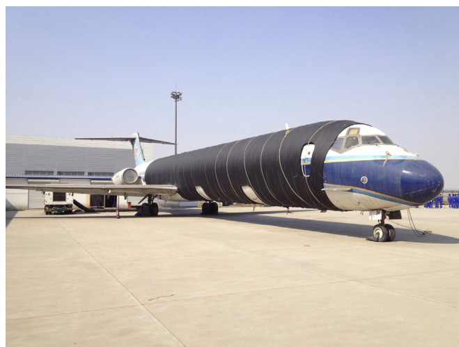
Fig. 1. Insulated MD-82 aircraft facility with envelope.
