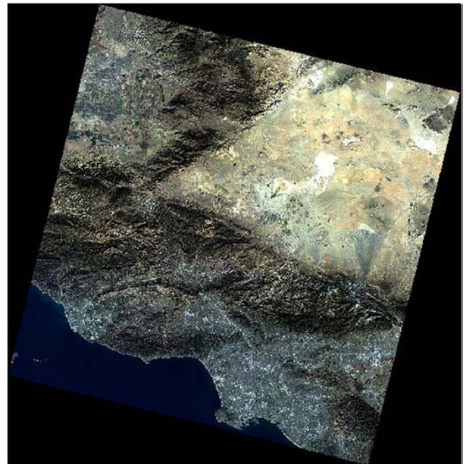
Fig. 2. A Landsat-8 image of 41/36 (path/row) acquired on 23 December 2013. The image is a color composite with Band 4 as red, Band 3 as green, and Band 2 as blue. There are no clouds. The image is used as a reference image. (For interpretation of the references to color in this figure legend, the reader is referred to the web version of this article.)
