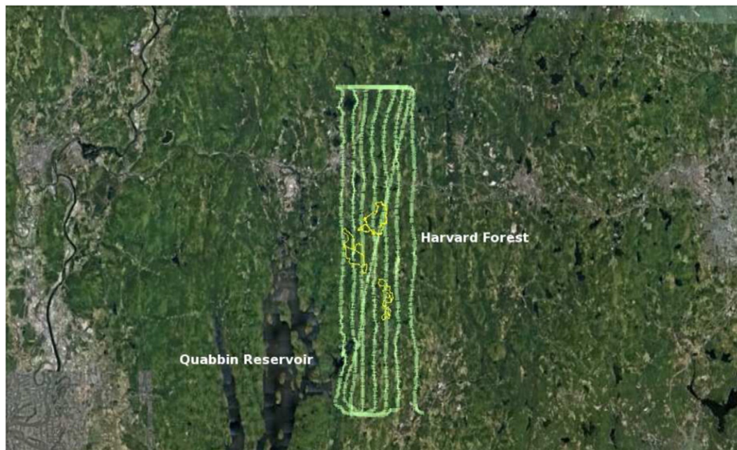
Fig. 1. The LVIS nadir track is highlighted by green lines while boundaries of the Harvard Forest are shown by the yellow lines. As the LVIS instrument flies along this track its beam scans up to 7° off either side to make a detailed height map of the area.
