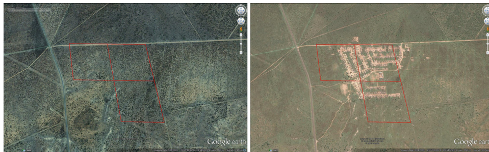
Fig. 1. Example of a new settlement development in the Limpopo province of South Africa. QuickBird image on the left shows the area being mostly covered by natural vegetation in 2003, whereas the QuickBird image on the right shows a new informal settlement in 2009 (courtesy of Google™ Earth). The red polygons show the footprint of three 500 m × 500 m MODIS pixels. (For interpretation of the references to color in this figure legend, the reader is referred to the web version of this article.)
