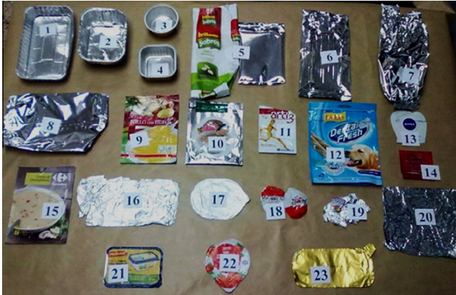
Fig. 1. The studied packaging samples (samples 1–4 – semi-rigid packagings; samples 5–15 – flexible with low Al content; samples 16–23 – flexible with high Al content).
