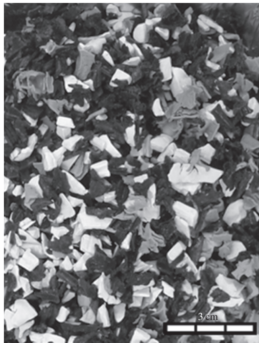
Fig. 1. Investigated sample coming from PVC window frame waste (1403 quality).
