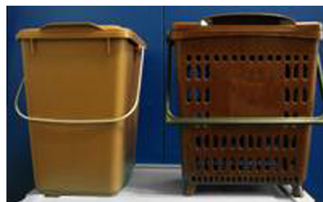
Fig. 1. Image of the bins used in this study. Non-aerated bin (nAB; left); Aerated bin (AB; right).
