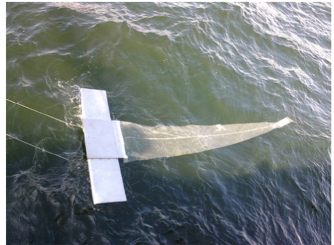
Fig. 2. Manta trawl deployed for sampling on the vessel side.
