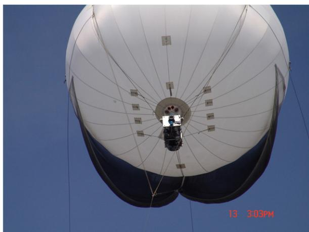
Fig. 1. Aerostat with sampling instruments and solids-laden aerostat sail.
