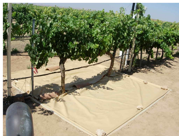
Fig. 1. View of the lysimeter with the waterproof canvas installed.
