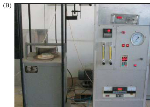
Fig. 2. Hollow fibre membrane system for oxygen production (A) flow chart; and (B) photo of the setup.
