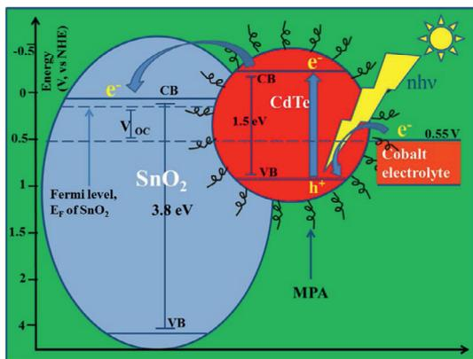
**Fig. 1.** Illustration of band alignment of materials used as photoanode ( $\text{SnO}_2$ ), sensitizer (CdTe), and electrolyte (Co electrolyte).
