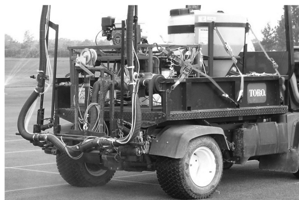
Fig. 3. Kamterter ULV turfgrass sprayer on a Toro Workman® 3200 applying treatments from an alternate angle in 2011.
