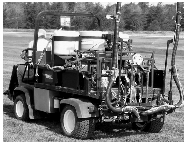
Fig. 2. Kamterter ULV turfgrass sprayer on a Toro Workman® 3200 applying treatments in a Kentucky bluegrass and perennial ryegrass mixture in 2012.
