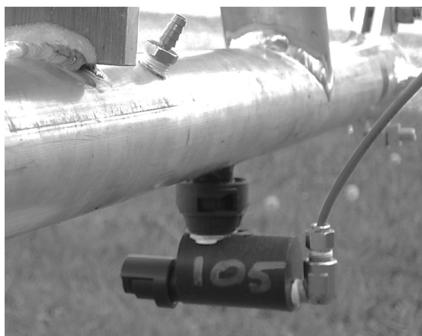
Fig. 1. Kamterter ULV Sprayer fixture attached to the spray boom. The fixture is attached to a dry boom where the air component of the system enters the mixing chamber (labeled 105) from above and is interacted with the liquid component which enters the fixture at the back.
