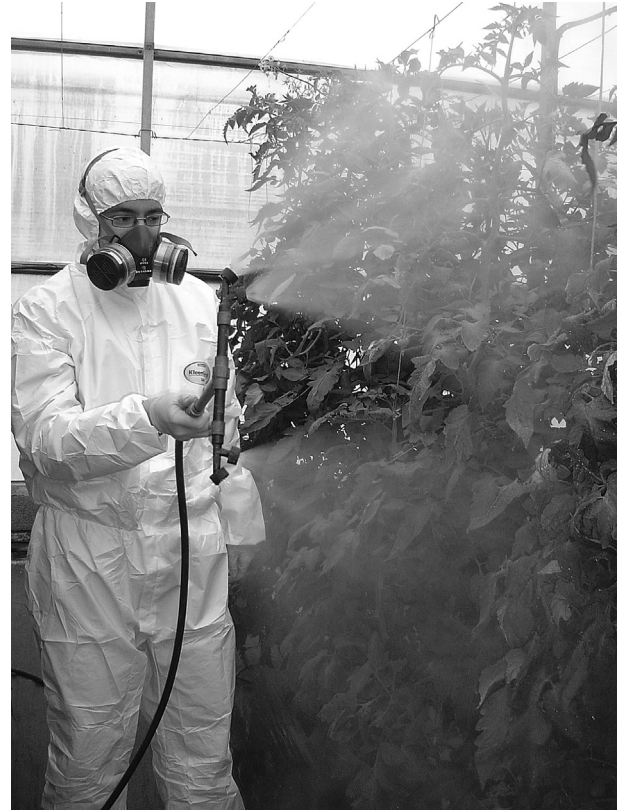
Fig. 2. Spray lance with four twin flat fan spray nozzles.
