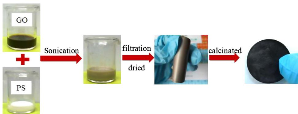
Fig. 1. Schematic illustration for the fabrication of 3DGF.
