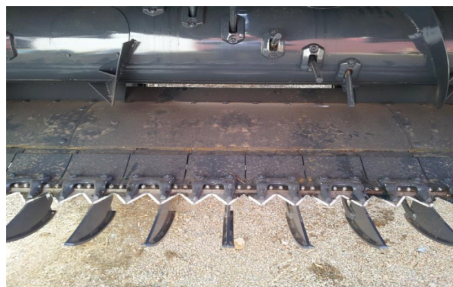
Fig. 1. Boot-shaped coulters of the self-leveling head.
