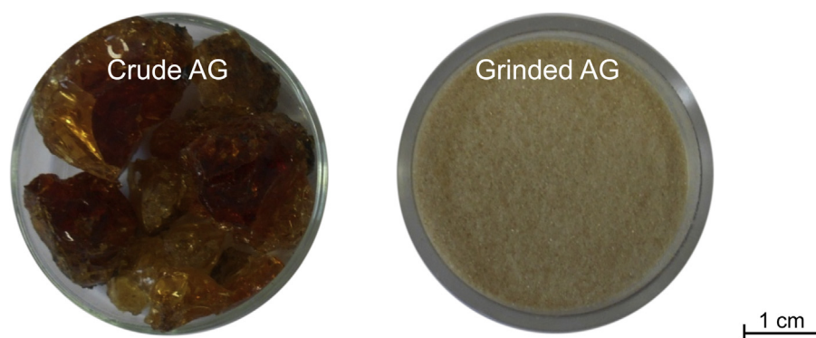
Fig. 1. Pictures of crude almond gum (collected from almond trees) and grinded almond gum after drying.
