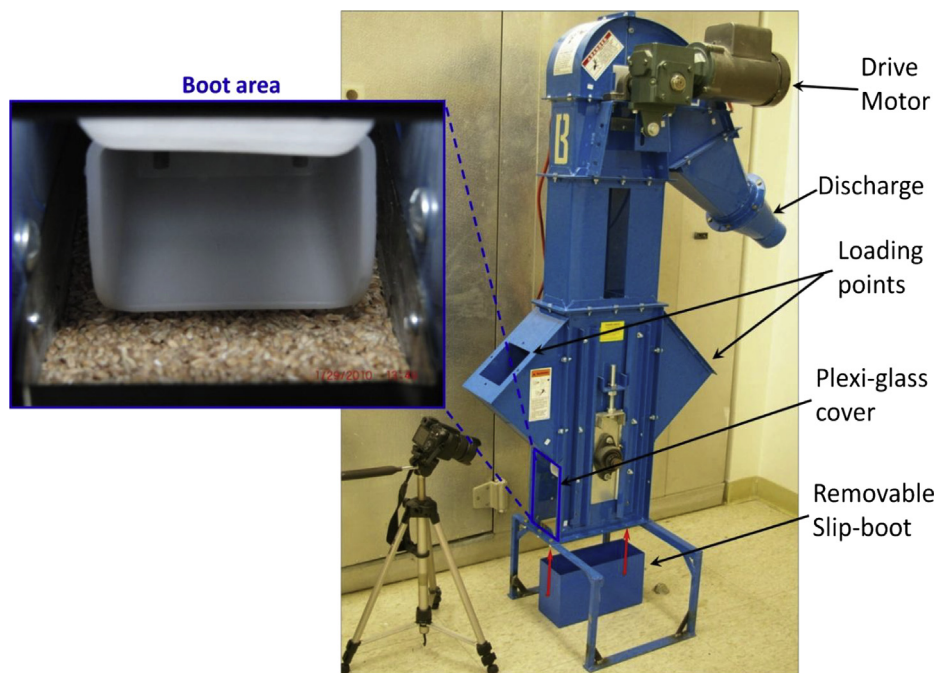
Fig. 1. Pilot-scale bucket elevator leg boot arrangement.
