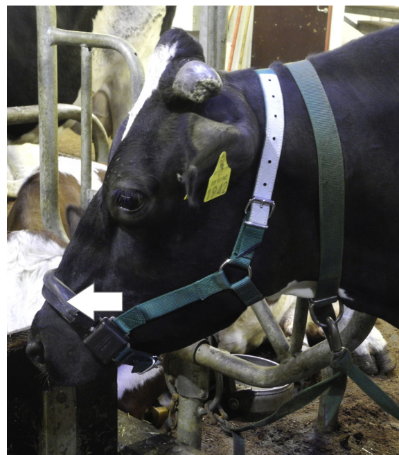
Fig. 1. A cow equipped with a RumiWatch noseband sensor. The pressure sensor is placed in the noseband of the halter (pointed by an arrow).
