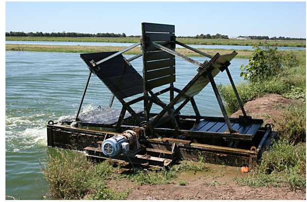
Fig. 1. The modular- and culvert based paddlewheel water circulator used in commercial split-pond systems.
