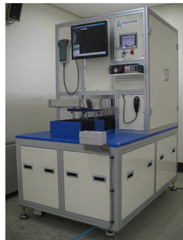
Fig. 1. Configuration of the automatic vaccine injection system for flatfish.
