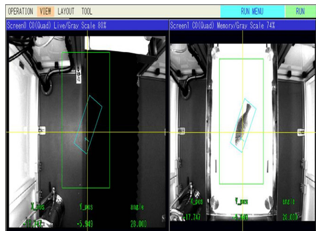
Fig. 2. Search scope (green line) and template (blue line) scope of the vision system.
