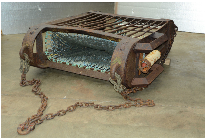
Fig. 1. The NIWA seamount sled, showing the net opening, bridles and break-away chains, and the location beacon mounted on the side (photo, NIWA).
