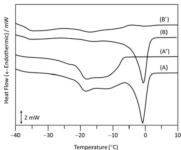
Fig. 2. DSC thermograms of (A) canola emulsion, (A') canola oil, (B) soybean emulsion, and (B') soybean oil during heating at a rate of  $2$  °C  $\text{min}^{-1}$ .
