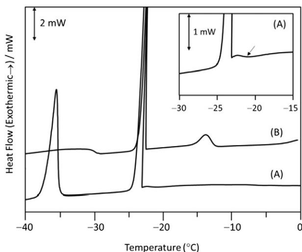
Fig. 1. DSC thermograms of (A) canola emulsion and (B) soybean emulsion during cooling at a rate of  $2$  °C  $\text{min}^{-1}$ . Insert presents magnified thermograms of (A) from  $-15$  to  $-30$  °C.
