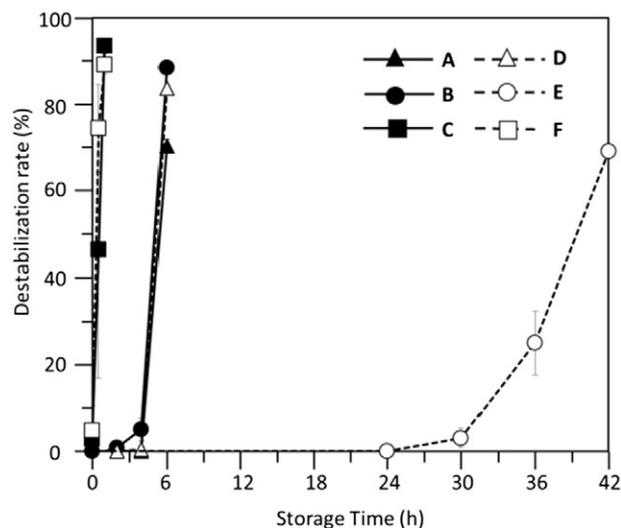
Fig. 3. Destabilization rate in the emulsions during storage from 0 to 42 h. (A)  $-15$  °C, (B)  $-20$  °C, and (C)  $-30$  °C of canola emulsions. (D)  $-15$  °C, (E)  $-20$  °C, and (F)  $-30$  °C of soybean emulsions. Error bars are S.D. ( $n = 4$ ).
