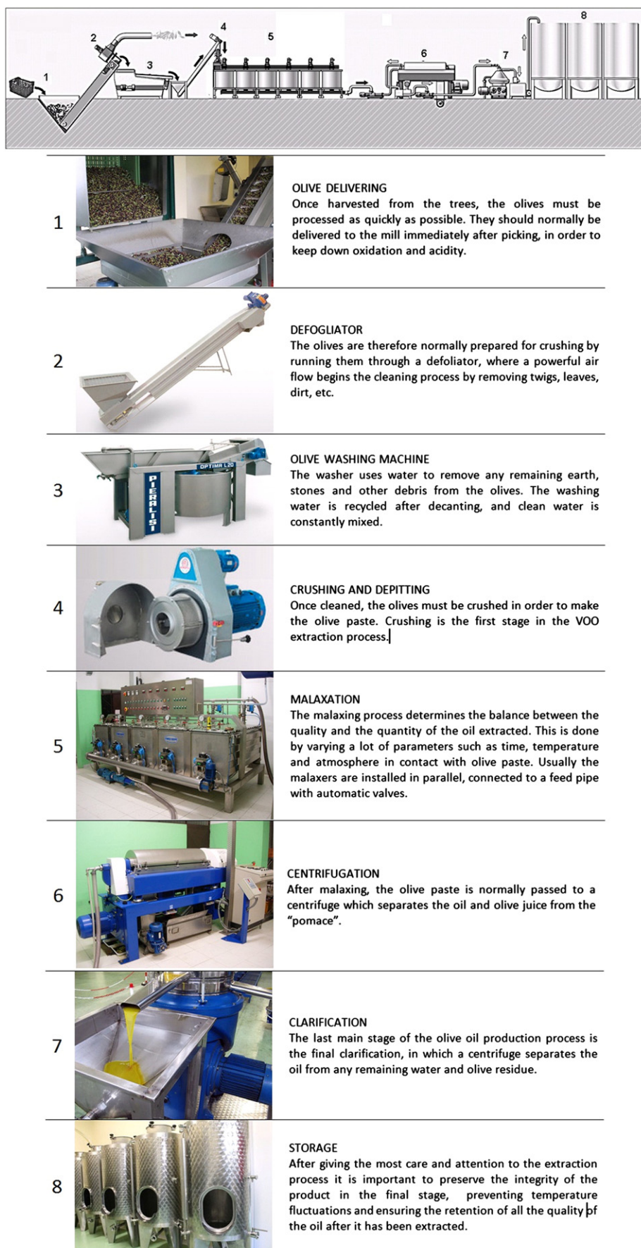
Fig. 1. Processes and machines composing an olive oil processing line: 1—Delivery system; 2—Leaf removal system; 3—Washing machine; 4—Hammer mill; 5—Batch malaxers; 6—Decanter; 7—Separator; 8—Storage tanks; (photos courtesy of Alfa Laval SpA, GEA Westfalia Separator Group, Pieralisi & Hakkı Usta).
