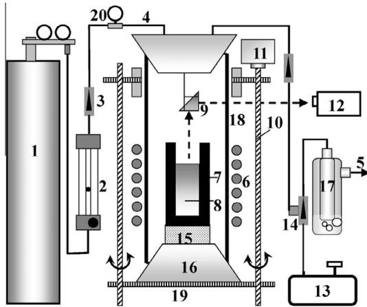
**Fig. 1.** Schematic of the induction furnace: 1. Ar gas tank; 2. gas flow meter; 3. two-way valve; 4. gas inlet; 5. gas outlet; 6. induction coils; 7. graphite crucible; 8. Al-Si solvent; 9. prism; 10. ball screw; 11. stepping motor; 12. infrared pyrometer; 13. vacuum pump; 14. three-way valve; 15. porous alumina holder; 16. silicone plug; 17. bubble checking; 18. quartz chamber; 19. stainless steel plate; 20. vacuum meter.
