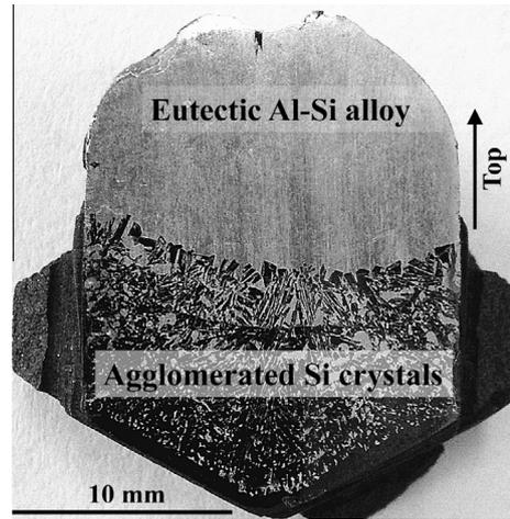
**Fig. 2.** A typical cross section of a Al-45 at.% Si alloy after electromagnetic solidification purification of Si.
