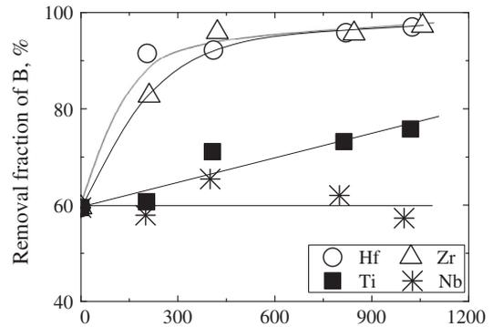
**Fig. 3.** B removal after electromagnetic solidification purification of Si with different additives.
