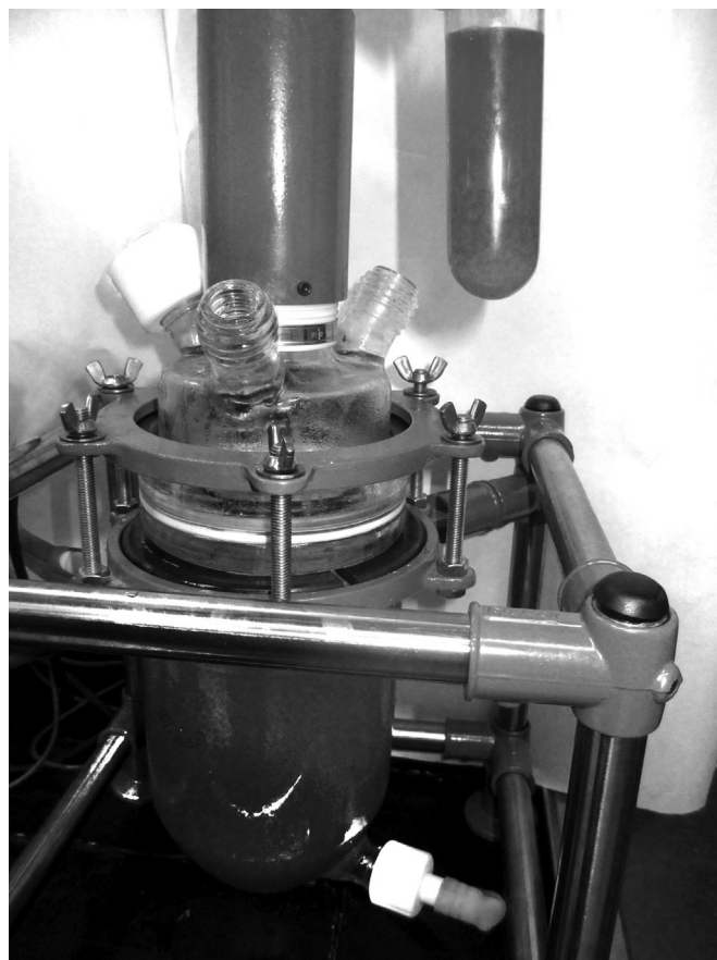
Fig. 1. Reactor used for the enzymatic degumming process of crude sunflower oil samples.
