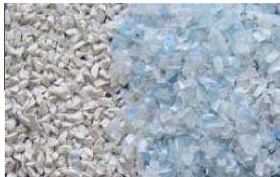
Fig. 3. Post-consumer PET (transparent-blue) and PVC (white) granules. (For interpretation of the references to color in this figure legend, the reader is referred to the web version of this article.)
