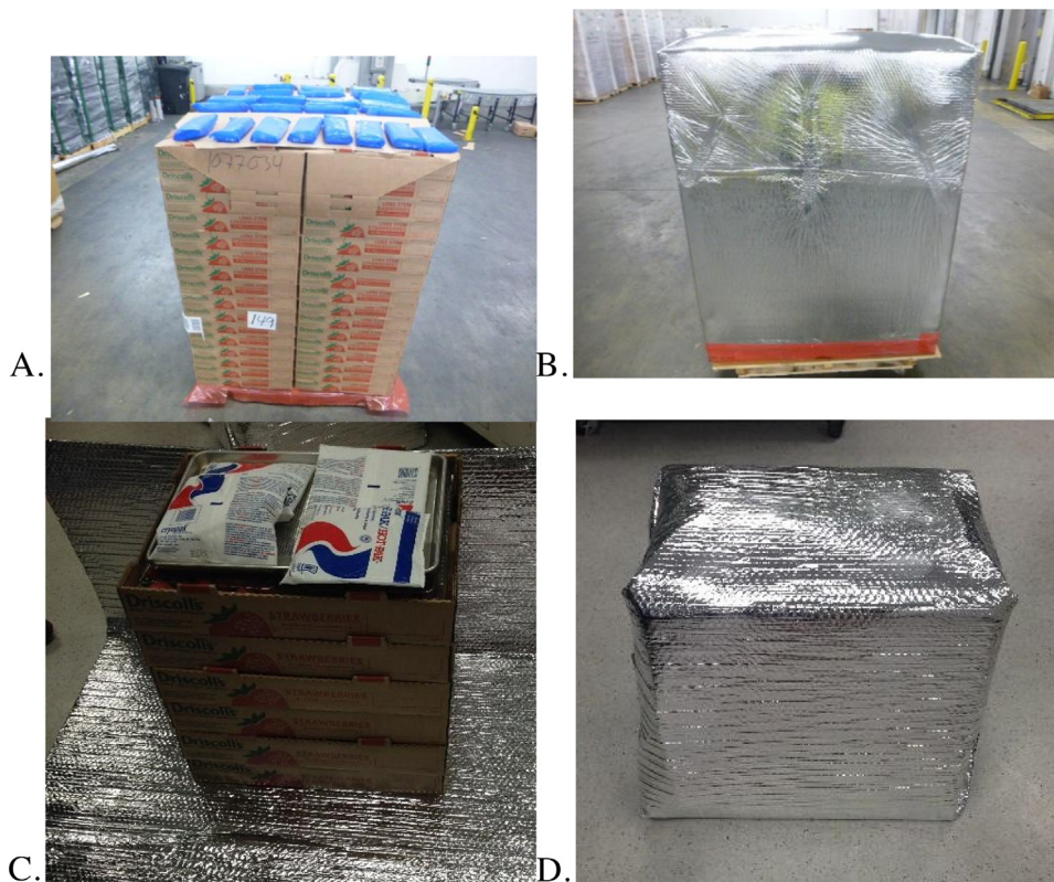
Fig. 1. Commercially air freighted strawberry pallets maintained cold (A) with ice packs (B) with ice packs and wrapped with insulated foil. Chapman University air freight simulation maintained cold (C) with ice packs (D) with ice packs and wrapped with insulated foil.
