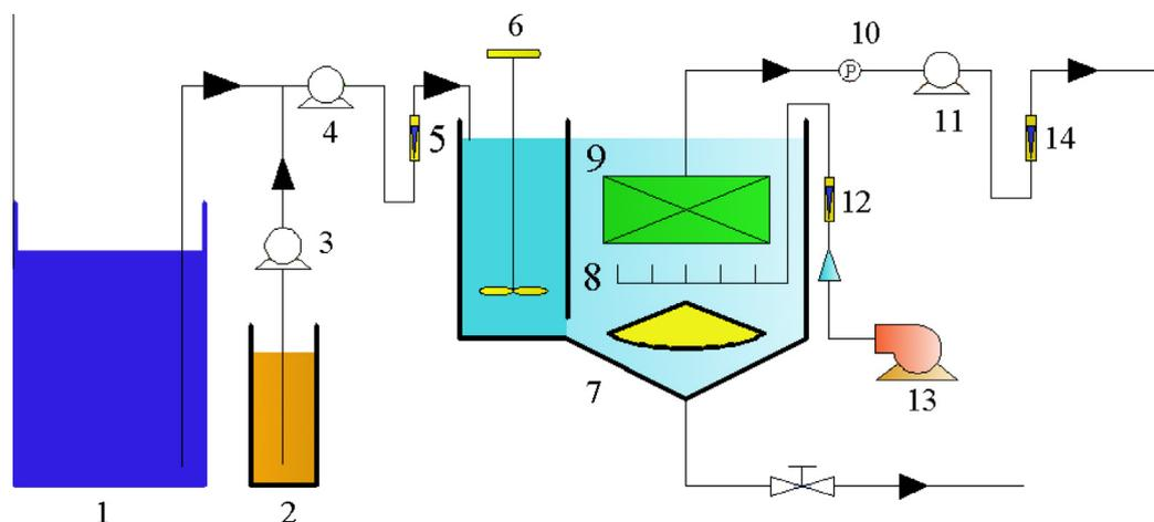
Fig. 1. Schematic diagram of the IMCR treating textile wastewater (1-feed tank; 2-coagulant tank; 3, 4, 11-pumps; 5, 14-liquid flowmeters; 6-stirrer; 7-IMCR; 8-air diffuser; 9-membrane module; 10-manometer; 12-air flowmeter; 13-air compressor).
