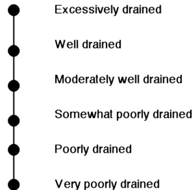
Fig. 1. Hypothetical soil drainage factor sequence represented as a simple chain or linear sequential graph.
