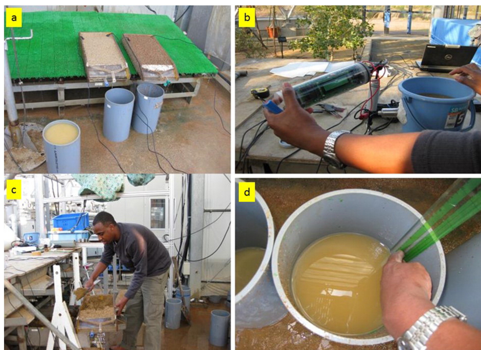
Fig. 1. Procedure of erodibility measurement using fluid energy method; setup of soil tank (soil exposure to rain) and runoff collector (a), SSC measurement using optical backscatter sensor (b), change soil sample (c) and runoff depth measurement (d).
