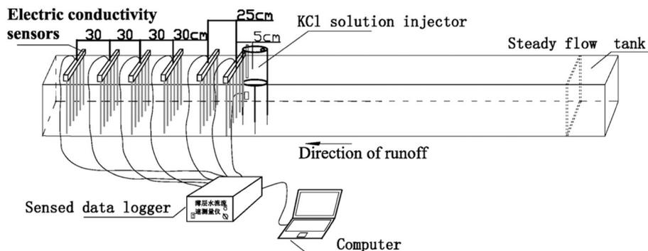
Fig. 2. The sketch of experimental equipment system.
