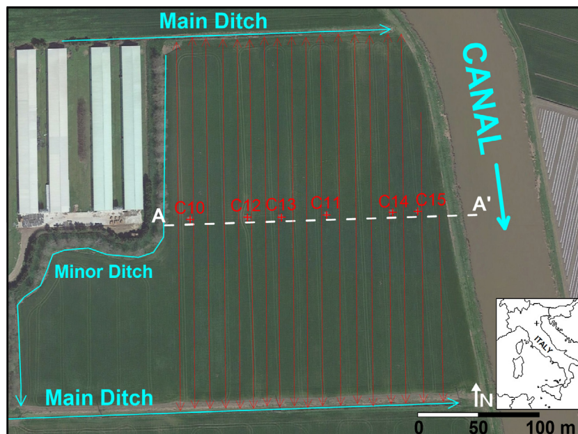
Fig. 1. Field site location with the main hydraulic features highlighted: tile-drains (red lines), ditches (cyan lines), monitoring wells (red crosses) and the model transect A–A' (dashed white line). (For interpretation of the references to colour in this figure legend, the reader is referred to the web version of this article.)
