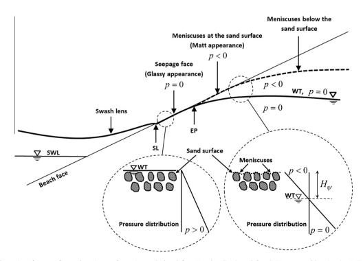
**Fig. 1.** Schematic illustration of seepage face and meniscuses formation on the beach face. SL = shoreline (swash front); EP = water table exit point; WT = water table; p = pore pressure;  $H_{\psi}$  = steady capillary fringe thickness. Solid and dashed lines represent the free surface and idealised meniscuses surface, respectively (after Cartwright et al., 2006).
