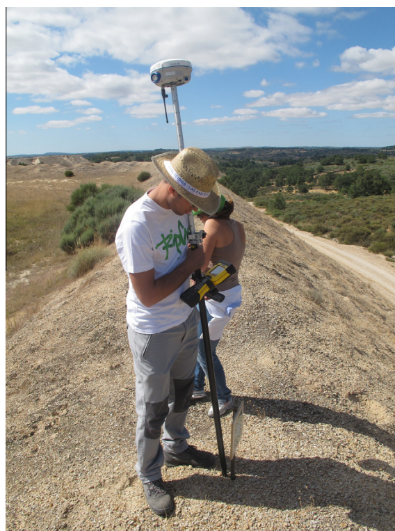
Fig. 1. GNSS-RTK (Real Time Kinematic) positioning.
