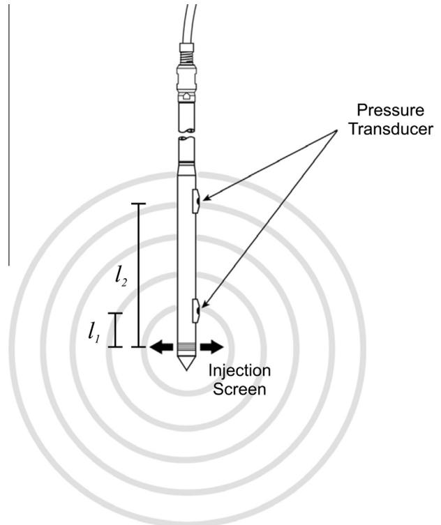
Fig. 1. Schematic sketch of the DPP probe (modified after Butler et al., 2007). Although not shown, the diameter of the probe increases slightly above the injection screen to diminish the potential for short circuiting flow along the probe.
