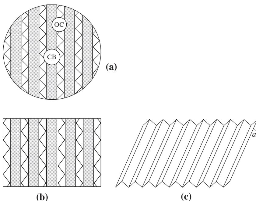
**Fig. 1.** Schematic representation of BH-1 type: (a) top view, (b) side view, and (c) one piece of the corrugated wire gauze sheets. OC and CB represent open channel and catalyst bag, respectively.
