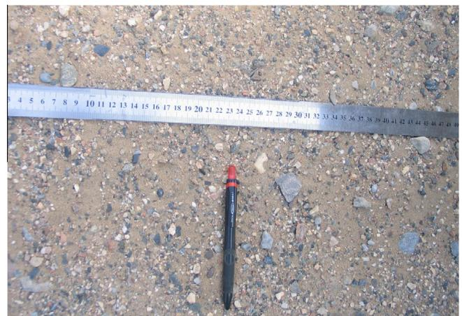
Fig. 2. The underlying surface of the wind tunnel floor.
