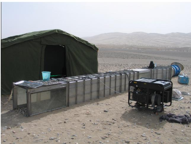
Fig. 1. The mobile wind tunnel.
