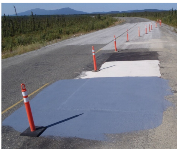
Fig. 1. Beaver Creek test site with surfaces from top to bottom: L-BST, Coldmix, Lafrentz and Nippo.
