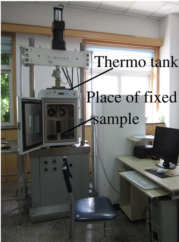
Fig. 1. Photograph of the uniaxial compression apparatus.
