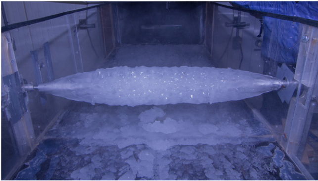
Fig. 1. Accumulated atmospheric ice on the rotating cylinder.
