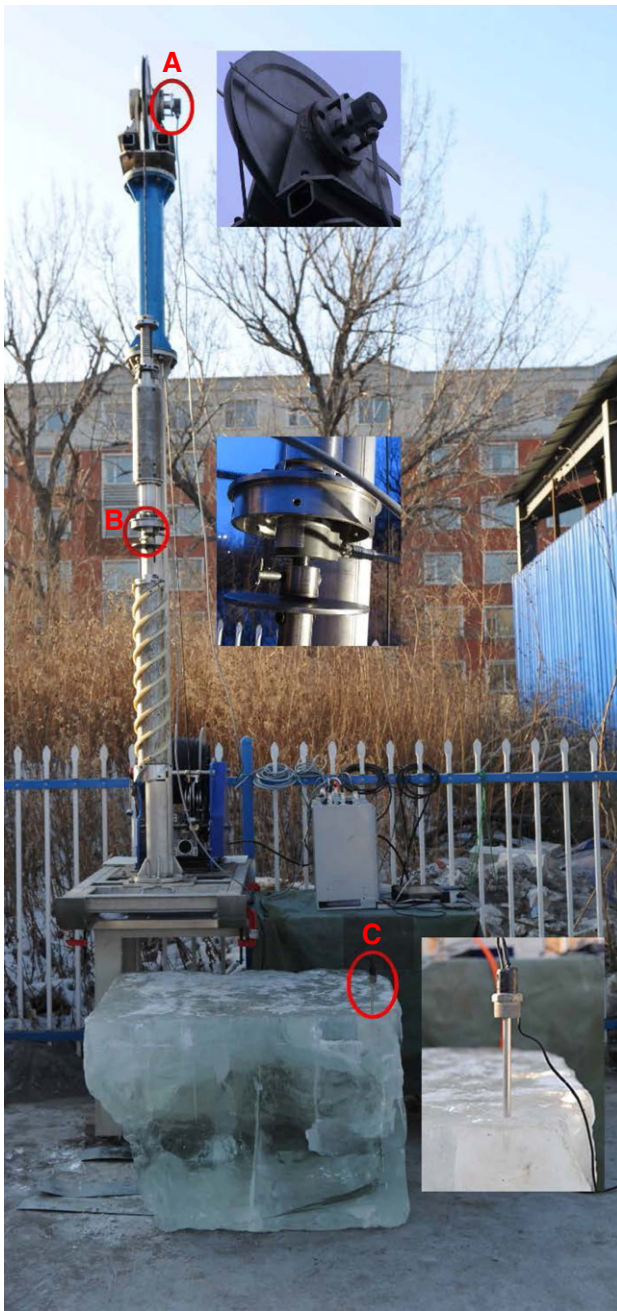
Fig. 1. Testing stand: A – encoder for the registration of the drilling depth; B – RPM sensor; C – thermometer fitted into the ice.
