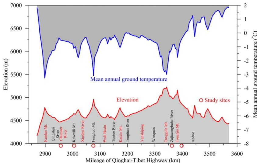
Fig. 1. Elevations and MAGTs along the Qinghai–Tibet Highway (after Zhao et al., 2010).
