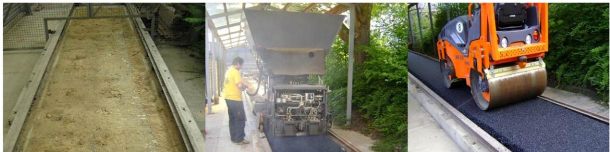
**Fig. 1.** Test track, paver and asphalt compaction.
