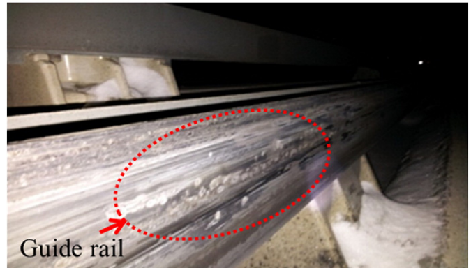
Fig. 3. Freezing at (a) collector shoe and (b) guide rail.
