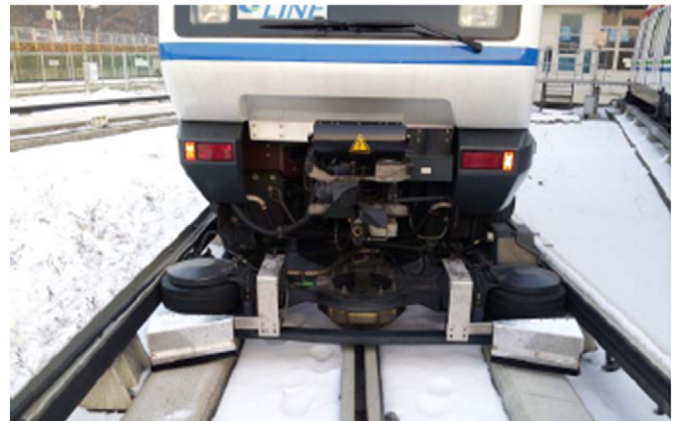
Fig. 4. Train nose with snow-removing brush.
